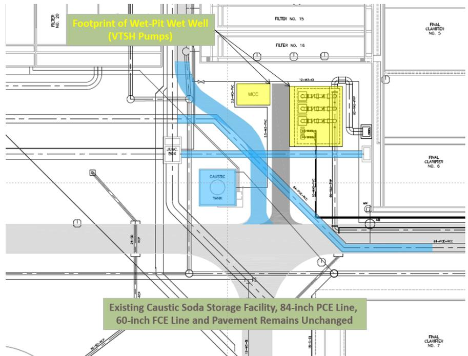
Figure 6. Footprint of a Vertical Turbine Solids Handling Pump Station (Wet Pit)
