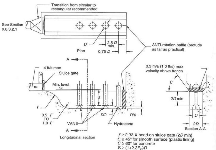
Figure 2. ANSI/HI 9.8 Pump Intake Design (1998)
