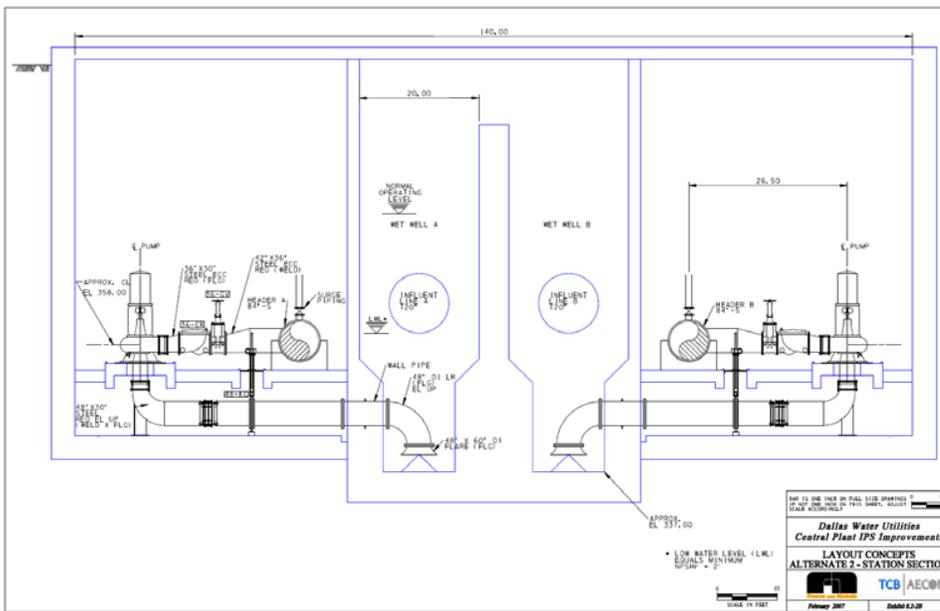
Figure 9. Layout for a Trench-Type Wet Well Dry Pit/Wet Pit Pump Station
