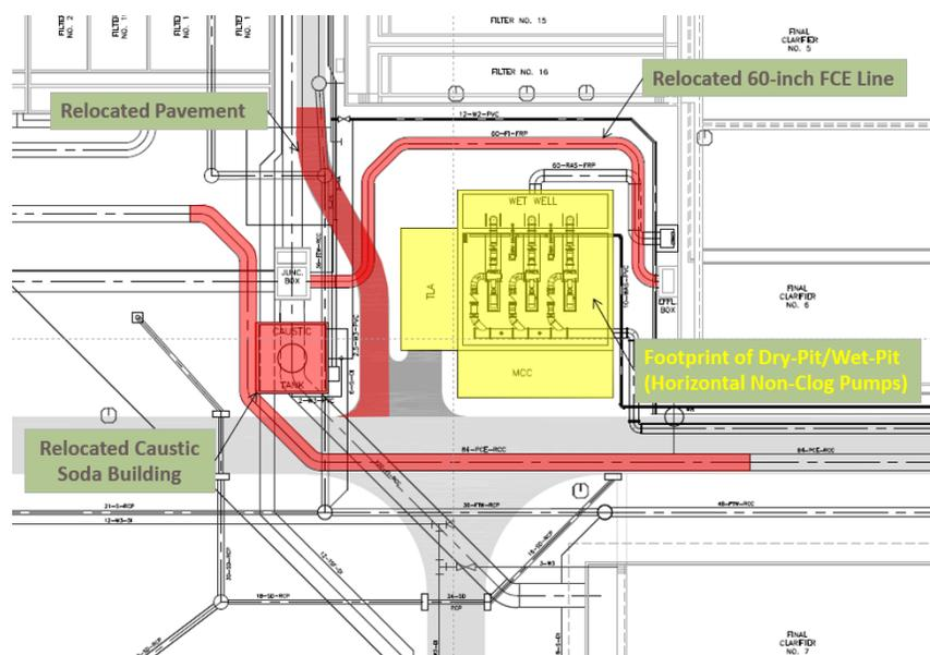
Figure 4. Footprint of a Horizontal Nonclog Pump Centrifugal Pump Station (Wet Pit/Dry Pit)
