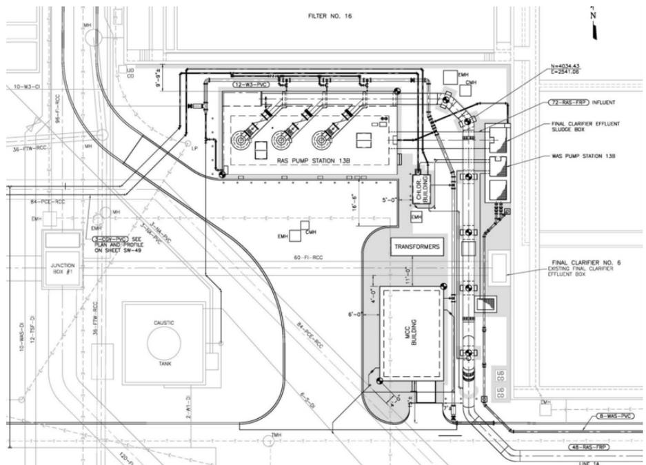
Figure 7. Footprint of a Vertical Turbine Solids Handling Trench-Type Wet Well (Wet Pit)
