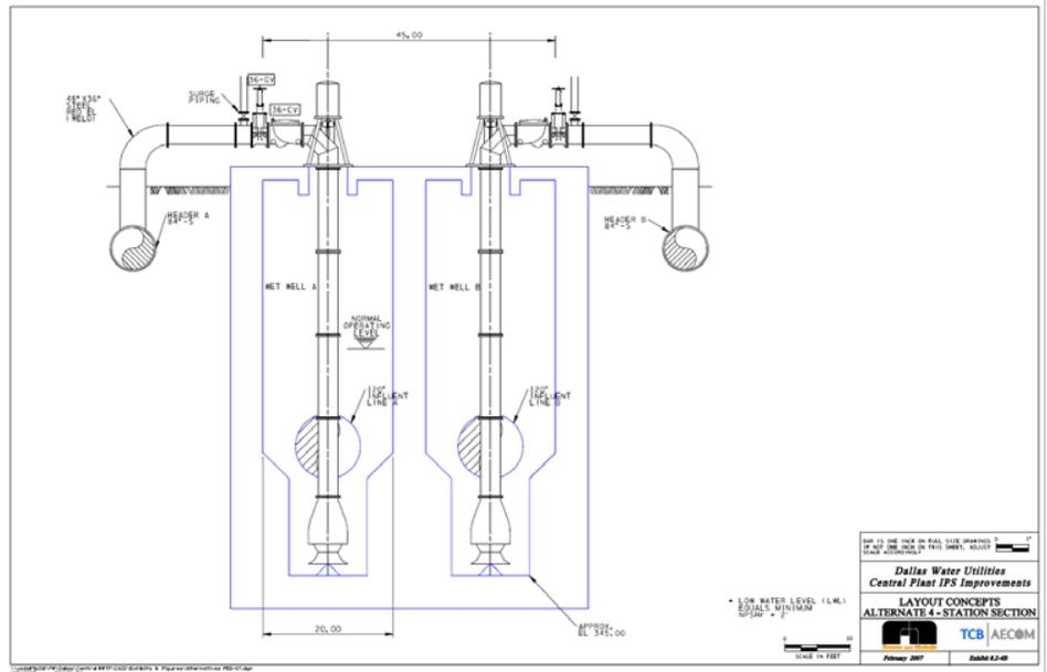
Figure 10. Layout for a Trench-Type Wet Well Vertical Turbine Solids Handling Pump Wet Pit Pump Station
