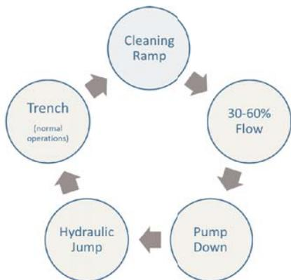
Figure 3. Self-Cleaning Phases of a Trench-Type Wet Well
