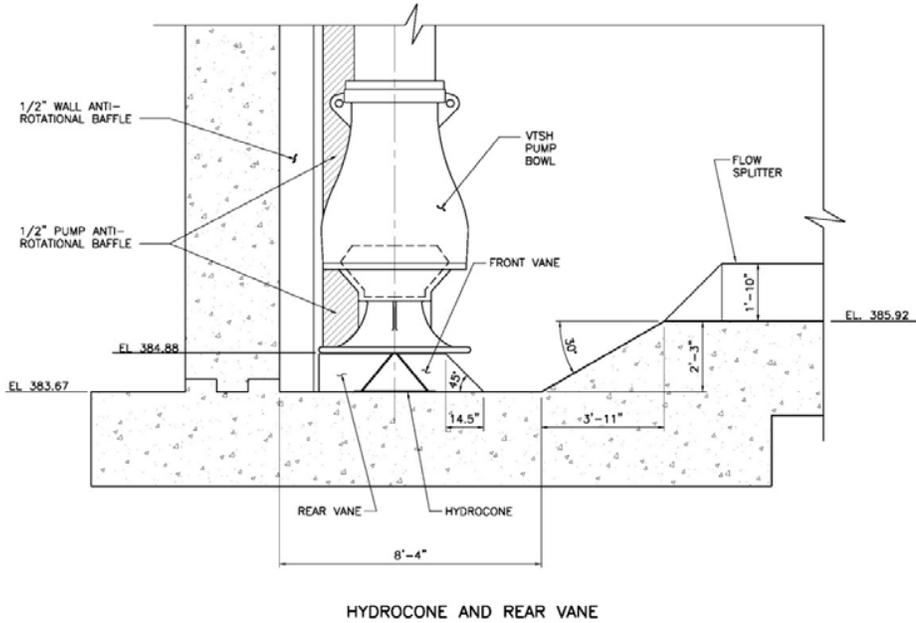
Figure 8. Hydrocone and Rear Vane Design in Pump Station 13B
