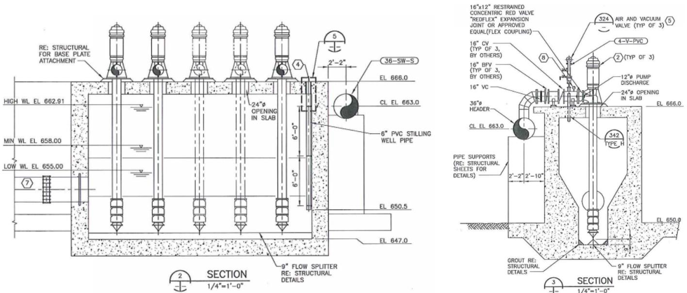
Figure 11. Section Views of Midlothian Water Treatment Plant Trench-Type Wet Well Pump Station
